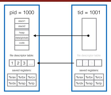
Under the hood, a thread gets its own "process control block" and is scheduled independently, but it is linked to the process that spawned it
